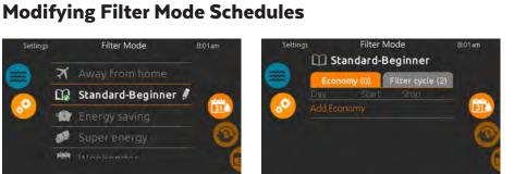
\*In economy mode, the set point will be reduced by 20°F - which means the heating system will not be engaged unless the temperature falls to 20°F below the hot tub's set temperature.
